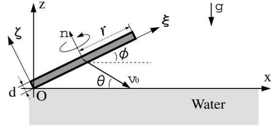
FIG. 2. An oblique water entry of a circular disk with incident angle  $\theta$  and initial velocity  $\mathbf{v}_0$ . The edge of the disk is taken at the origin of the coordinates at  $t = 0$ . The radius and thickness of the disk is  $R$  and  $d$ . The angle between the disk and water plane is  $\phi$ .
