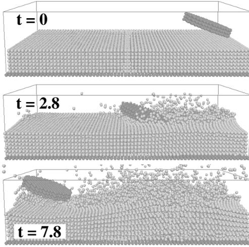
FIG. 1. Snapshots of the SPH simulation of a disk-water impact with  $\phi = 20^\circ$  and incident angle  $\theta = 15^\circ$ . Specific gravity of the disk  $\sigma = 2.7$ . The unit of time is scaled with  $r/v_0$ . The number of fluid particles  $N = 18837$ .
