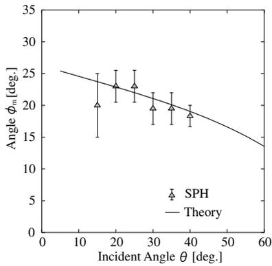
FIG. 4. Relation of incident angle  $\theta$  and the angle  $\phi_m$ . The SPH simulation is performed with  $\sigma = 2.0$ . The solid line is obtained numerically seeking the minimum of Eq. (7).
