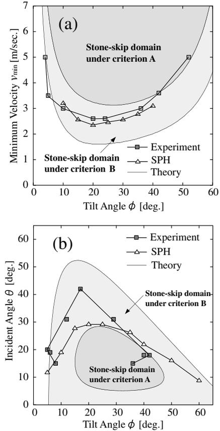
FIG. 3. A comparison of the stone skipping domains obtained from the experiment ([12]), SPH simulations, and our theory. (a) The stone skipping domain in the  $(v, \phi)$  plane for a fixed  $\theta = 20^\circ$ . (b) The stone skipping domain in the  $(\theta, \phi)$  plane for a fixed  $v = 3.5$ [m/s]. The boundary of the stone skipping domain under the criterion *A* in each graph are numerically drawn and those of *B* are the plot of Eqs. (7) and (8), respectively.
